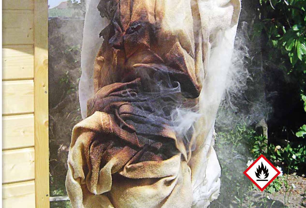
Cloth soaked with Base Oil: Condition after approx. 3 hours under ideal conditions: 30°C air temperature, no wind and direct sunlight
