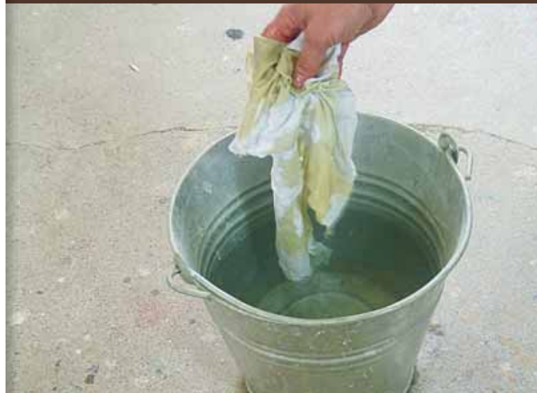
Cloth soaked with Base Oil: Condition after approx. 3 hours under ideal conditions: 30°C air temperature, no wind and direct sunlight
